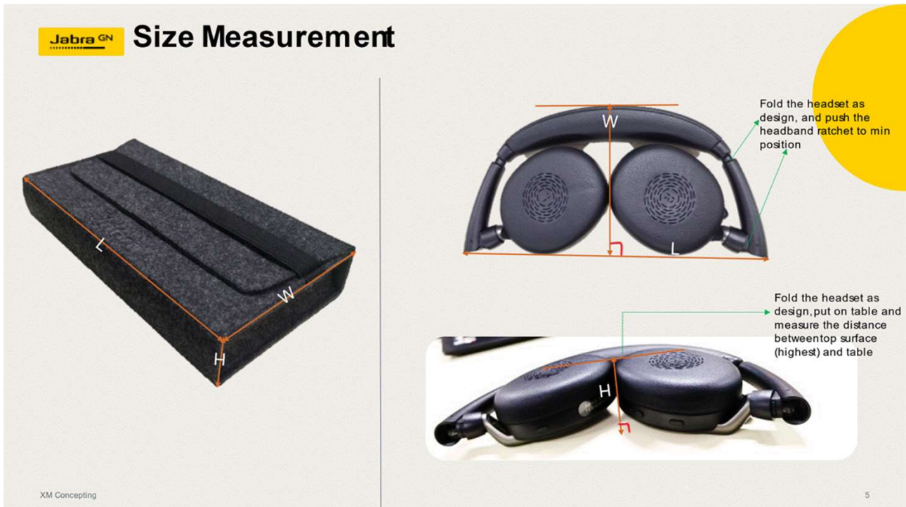
Figure 1 - Size measurement procedure – the left-hand side describes measurement with pouch, right-hand side without.
