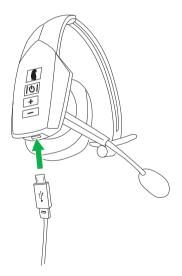
While charging, the LED indicator shows the charging status. Red indicates the headset is charging. Blue indicates the headset is fully charged.
