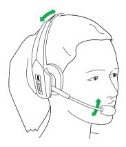
Position the microphone close to the corner of your mouth. Adjust the headband length so that the headset fits your head comfortably.
