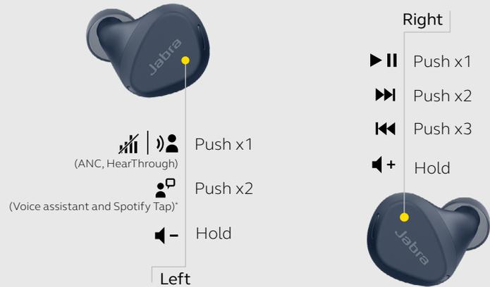
Tap both buttons simultaneously to power off
