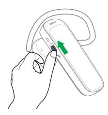
2. Simultaneously press and hold (6 seconds) the **Answer/end** button and the **Volume +** button, and then release the buttons.
