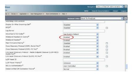
Under the tab "Wideband Headset UC Control", the option "Enabled" must be selected for each terminal phone.
