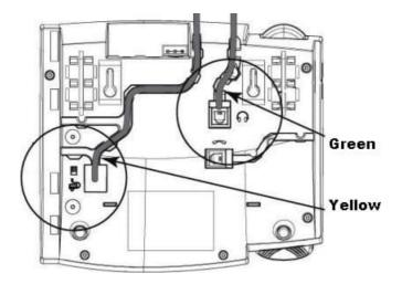
Insert the RJ10 plug (marked green) into the "headset" socket and the RJ45 plug (marked yellow) into the socket for the expansion module/ expansion modules.
