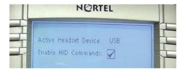
You must enable Headset option on the telephone. Services /Telephone Options / On Hook Default Audio Path / Headset Enabled. When phone is idle, customer must press "Services" button twice quickly. Then there will be one of two options: If they see "password", enter default: "26567\*738" then follow the below info. If they see "Preferences", then they choose "3" for headset/active headset device and select "USB". Be
