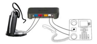
Please note that full functionality is only available when all the colormarked parts of the cables are inserted into the EHS adapter, see photo.
