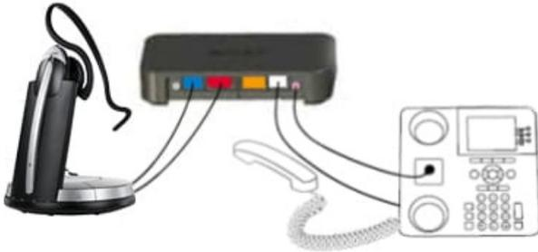
Please note that full functionality is only available when all the color-marked parts of the cables are inserted into the EHS adapter, see photo.
